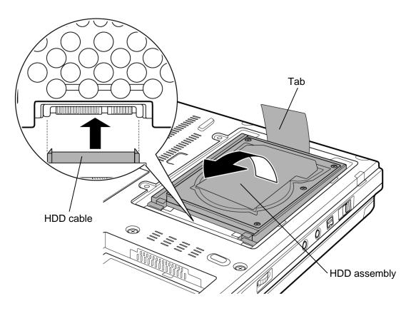
Figure 4-7 Removing the HDD assembly
